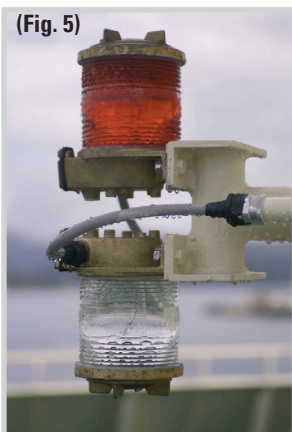
Fig. 5: Recommended mounted double tiers and single lanterns.
