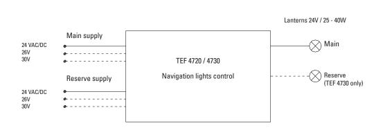
Compensation of voltage drop in long cables.
