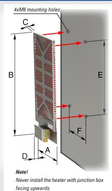
4xØ6 mounting holes on the backside of the heater.
