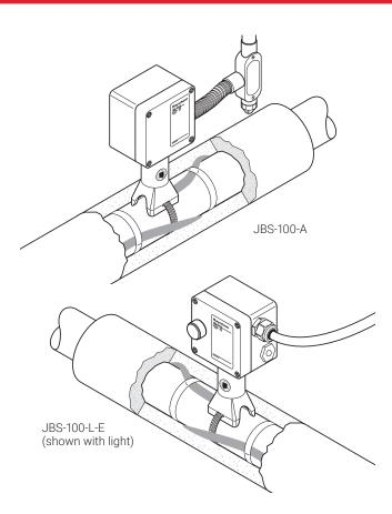
The nVent RAYCHEM JBS-100 kit is designed to connect power to one nVent RAYCHEM BTV, QTVR, XTV, KTV or VPL industrial parallel heating cable. It is approved by FM, CSA, and PTB for use in hazardous locations.
