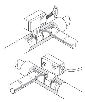
The nVent RAYCHEM JBM-100 kit is designed to connect power to up to three nVent RAYCHEM BTV, QTVR, XTV, KTV, or VPL industrial parallel heating cables and is approved by FM, CSA, and PTB for use in hazardous locations.
