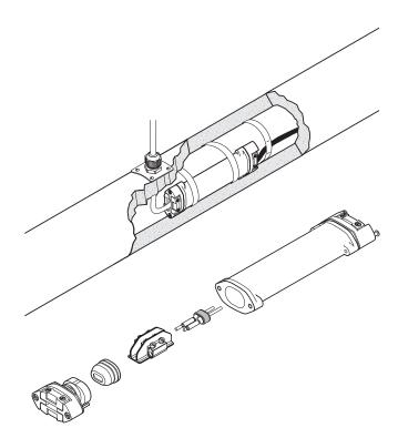
The nVent RAYCHEM C-150-E is a cold applied low profile power connection. The kit enables in line connection of nVent RAYCHEM industrial heating cables, BTV, QTVR, XTV and KTV, to a flexible power cable. It can be used in applications with temperature ratings from  $-50^{\circ}$ C to 215°C. It is approved for use in hazardous areas.
