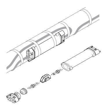
The nVent RAYCHEM S-150 is a cold applied low profile splice for in-line connection. This universal kit fits with all nVent RAYCHEM industrial heating cables, BTV, QTVR, XTV and KTV, meaning simplified product selection and reduced inventory to stock. It can be used in applications with temperatures ranging from  $-50^{\circ}$ C to  $215^{\circ}$ C. It is approved for use in hazardous areas.
