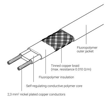
The nVent RAYCHEM 30TLT2-CT self regulating heating cable is designed for winterization applications in non-hazardous marine markets, such as under-deck heating of metal walkways on vessels. This heating cable demonstrates excellent thermal performance, long service life, easy installation, and low operating costs.
