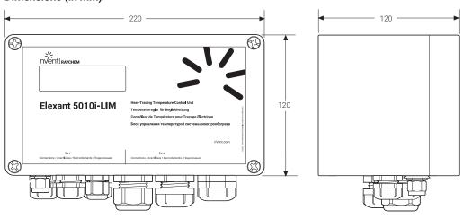
Sample shown is Elexant 5010i-LIM. Gland included in scope of delivery - 1 x M25 x 1,5
