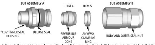
1. Separate the gland into two sub-assemblies, A and B, by unscrewing the body (2) from the entry item (1). Note that items (4) and (5) are loose items.
