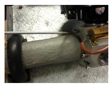
Connect the wires in parallel (red cable with red)
