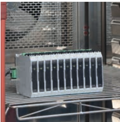
Ageing test for ISpac in the temperature test chamber
